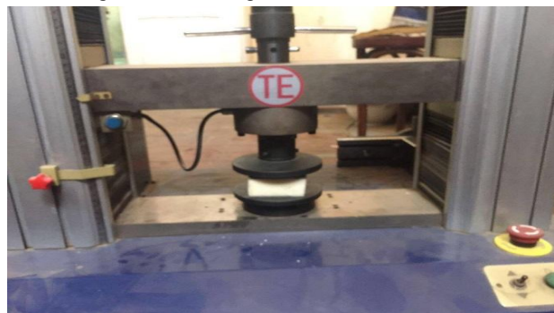
Figure 7 compression test for test specimen using Universal Testing Machine
