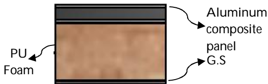
Figure 5 Al-C sandwich panel (Hybrid-PU sandwich composite)
