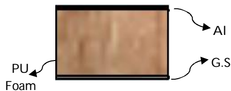
Figure 3 Al sandwich panel (Metallic-PU sandwich composite)
