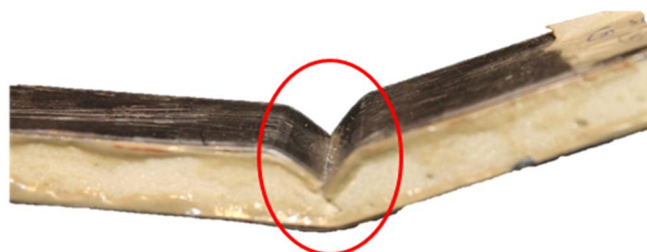
Figure 26 failure pattern in G.S(0.5) C(10) G.S(0.5)
