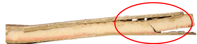
Figure 29 failure pattern in G.S(0.5) C (10) F.G(3)
