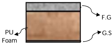
Figure 4 F.G sandwich panel (Hybrid-PU sandwich composite)
