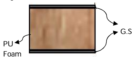
Figure 2 G.S sandwich panel (Metallic-PU sandwich composite)
